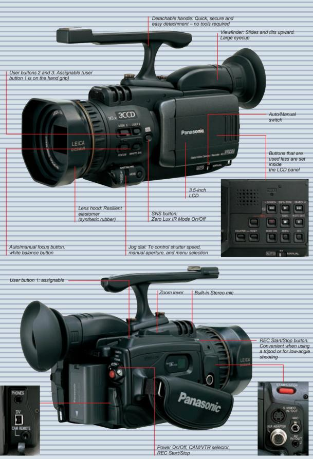
Terminals for headphone, digital interface, and camera remote. Split cover allows access to headphone terminal only. S-Video In/Out, Mic In/Out, AV In/Out, XLR Adapter terminals (XLR Adapter can be used with cover attached)
